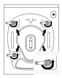
Pull out the bolts together with the coloured plastic spacer, (the screws that have been removed from the machine should be kept in case the machine needs to be used in future).
